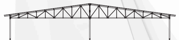
Drop Ceiling with Internal Column
