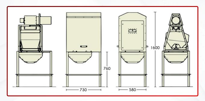
The mechanical weigher give us an accurate and reliable method of weighing a continuous feed flow passing through the weigh chamber to measure up to 100 tips per hour with range of 6 to 12kg per batch.
